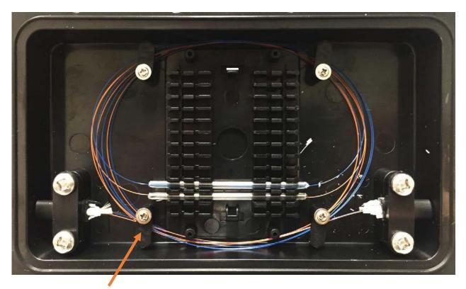
The four fiber retention wings are positioned to keep the fibers captive to the base of the DFR100 so the fibers do not fall or spring out of position.
